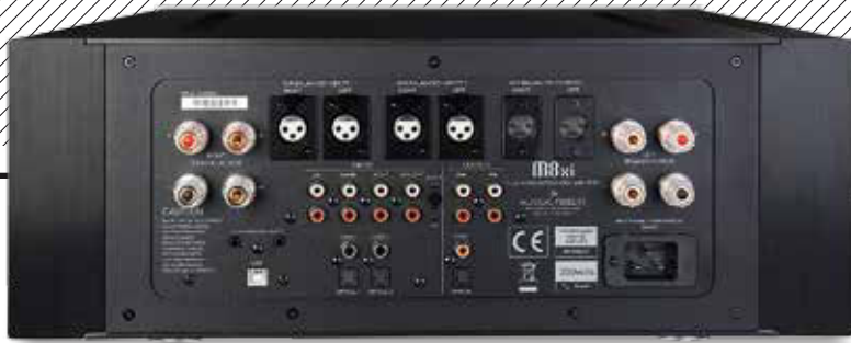
ABOVE: Five line ins (three on RCA, two balanced on XLRs), USB-B and pairs of coax/optical digital ins are joined by balanced and single-ended pre outs (XLR/RCA), one fixed line out (RCA) and coax/optical digital outs. There are two sets of floating (live negative and positive) 4mm speaker outlets per channel for easy bi-wiring
